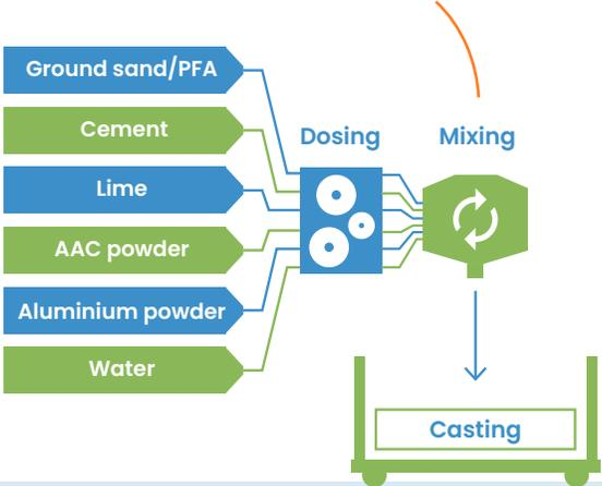
The hydrogen gas foams and increases the volume of the raw mix creating bubbles up to 3 millimetres in diameter, causing it to rise like bread dough.
